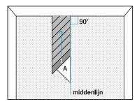
**3.** Lay guide piece A with 45° corners along the centre line, making sure that guide piece A is not on the glue. Then lay the first row of strips on the glue. Begin with the starting strip and then install the strips above the starting strip.
