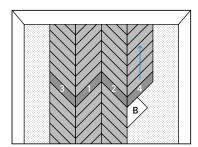
8. Then install the row on the right-hand side using guide piece B.
