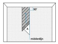
**3.** Lay guide piece A with 45° corners along the centre line, making sure that guide piece A is not on the glue. Then lay the first row of strips on the glue. Begin with the starting strip and then install the strips above the starting strip.
