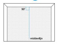
1. Identify the centre of the room (viewed from the starting wall) and make a line at right angles to the starting wall using a chalk line. This is the centre line.
