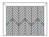
**9.** Continuously check that all strips are perfectly straight and the angles are always 90°. Keep repeating this sequence until the floor is finished.
