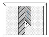
**6.** When the starting row is properly fixed, continue with the second row, to the right of the starting row. Start again with the starting strip, using guide piece A. Again, work first upwards and only then downwards.
