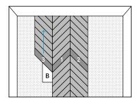
7. Continue with the row to the left of the starting strip, using guide piece B with the 135° angle. Again, work first upwards and then downwards.
