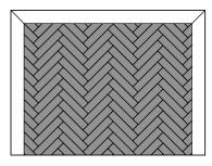
**7.** Remove the strips stuck together with tape and lay the floor close against the starting wall.
