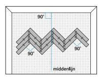
**2.** Lay two or three rows of strips against each other. Make sure that the corners are exactly 90° and fasten the strips tightly together with tape.
