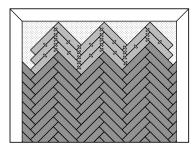
**6.** Repeat this procedure to the left and right of the laid starting strip. Continuously check that all angles are still 90°.
