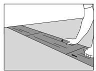
**2.** Lay the panels without stress and adjoining each other. When laying large tiles, follow the direction of the arrows on the back.
