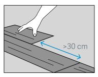
**5.** For the second and each subsequent row, take a new panel and decide how large the panel should be (or use a piece left over from one of the previous rows). With boards, make sure that the joint of the short side is at least 30 cm from the joint of the short side of the previous row; and at least 20 cm in the case of tiles.
