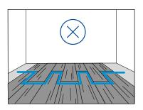
**4.** For a natural look, we recommend that the piece left over from the first row should not be used as the first piece of the second row. Avoid having a recognisable, repeating distance between the panels, which creates a kind of staircase effect. Boards are installed randomly and tiles can be installed in a straight line, in a half-brick bond or in an irregular bond.
